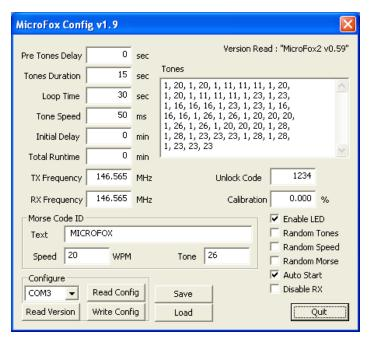
The default settings that appear when the configuration program is started are recommended for a basic hunt with the BFoxCon transmitting tones for 15 seconds, and then a Morse code ID. It then will stop transmitting, and repeats every 30 seconds. The only setting users must change is the Morse Code ID text to be their assigned amateur radio callsign.
