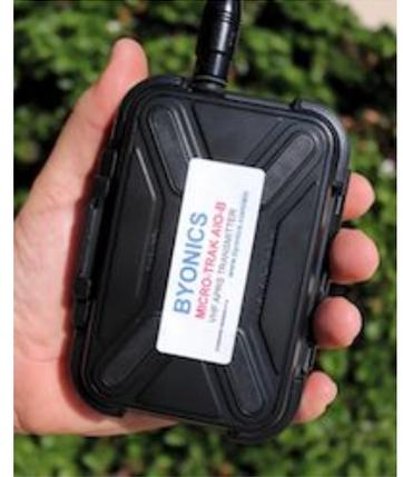
The MT-AIO-B is computer programmable and frequency agile over the entire 2 meter ham band in 5 KHZ channel steps. The device is rugged and intended for operation using alkaline AA batteries for ground operations or Energizer “Ultimate Lithium” AA batteries for high altitude and/or cold temperature operations. The MT-AIO-B sends voltage and temperature telemetry in the MIC-E format and may be viewed graphically on websites like aprs.fi.
