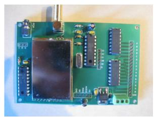
The Micro-Trak **DTMF** Receiver/Decoder is integrated an programmable VHF receiver, designed primarily for remote control applications. The receiver may be set to any 2 meter amateur radio frequency (in 5 KHZ channel steps) via a terminal program and a standard, Kenwood style (2.5mm, three conductor, plug) programming cable. (Available from Byonics) The decoder will decode all standard DTMF touchtones, from your VHF transmitter, and set
