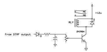
In this example, an R/C timer is added to the circuit. This will keep the relay activated for a time period determined by the value of the electrolytic capacitor and the potentiometer. This can be used to allow (for instance) one DTMF tone to temporarily activate the relay, which can then be utilized to pass any other output, allowing a simple "password" protection, since the second "command" tone may only be passed before the relay timer is active.
