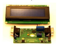
red stripe on the ribbon cable should be nearest the center of the PCB. The ribbon cable can be replaced with a longer cable if desired, up to 15 feet.
