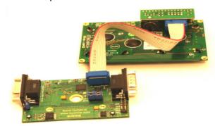
This adapter can also be used with the kit version of the TinyTrak4 with through hole components. There is not a connector for connection, so instead the ribbon cable should be soldered directly to pins on the underside of the TinyTrak4 circuit board, as shown below.
